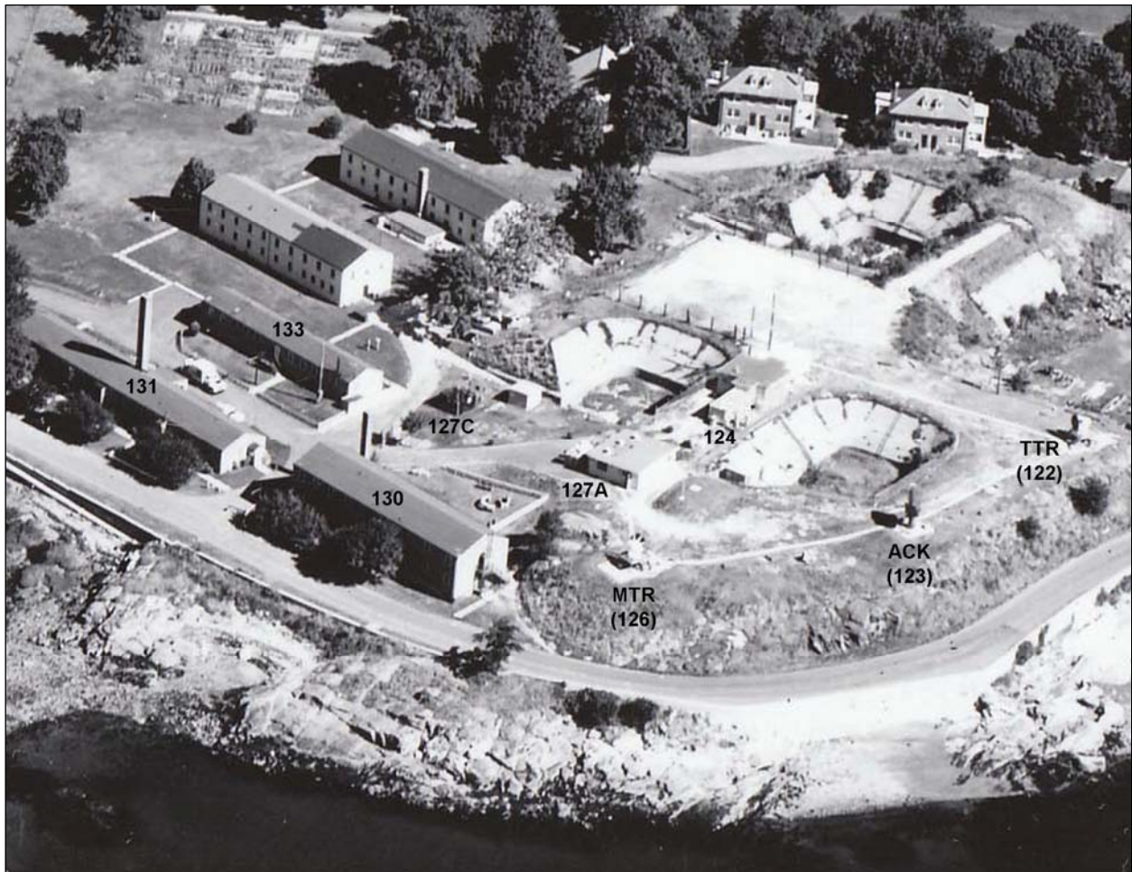
Figure 1. High angle oblique aerial photograph of Davids Island, ca. 1958, detail. View north. Labels have been added to this version of the image to indicate buildings and structures included in the Nike Battery NY-15 IFC Area. The battery's three radar sets are visible in this image and are labeled as follows: MTR—missile tracking radar; ACK—target acquisition radar; and TTR—target tracking radar. Building 124 is near the center of the image. Original from Record Group 291, National Archives, New York, NY; digital copy from Fort Slocum Alumni and Friends Collection, Michael A. Cavanaugh, Los Angeles, CA, custodian.
